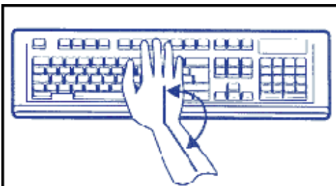
Fig. 1 Hazardous side bending of the wrist.
